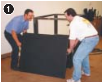
1 The lift is disassembled into six components, starting with the ramp.
