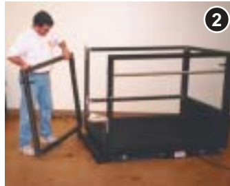
2 Next, the two gates are removed.
