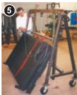
5 The base is easily raised onto the base relocator hoist.
